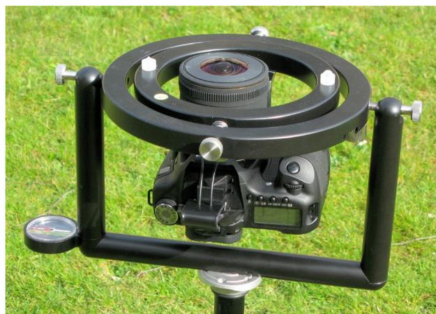
Digital SLR camera in the SLM10 Self-levelling Mount
